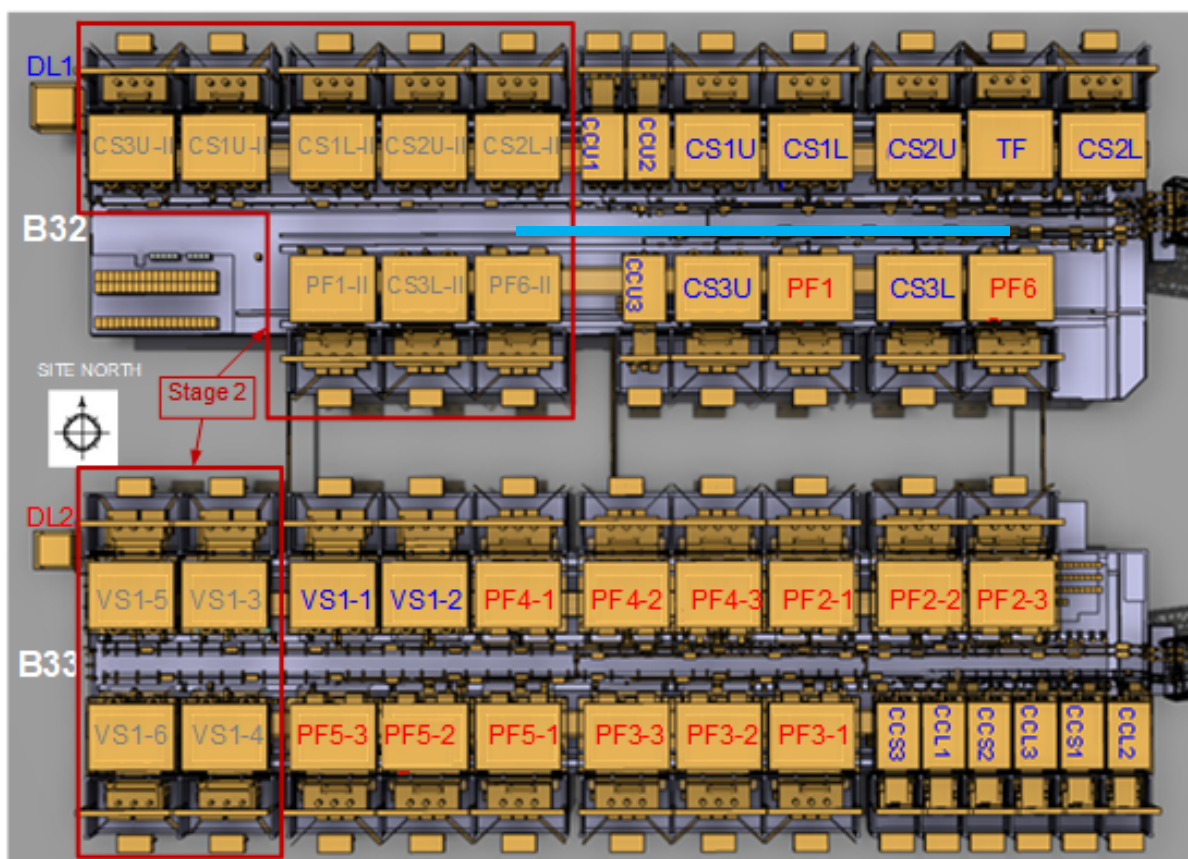
Figure 3-4 Layout of main coil power supplies in B32 and B33
