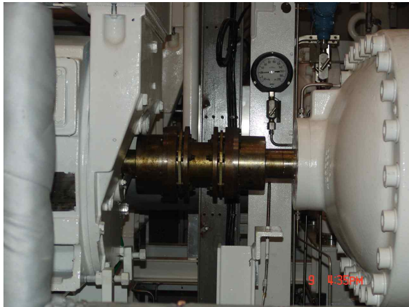
(a) motor-compressor coupling
