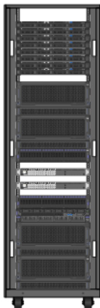
ITER 2 X V7000 8 X NSD Server 2 X 60 TB NVME 4 X Expansion shelves 4 PB
