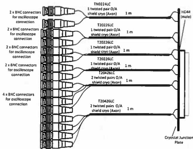
Run Electrical testing separately for TN0224LC, T20226LC and T20426LC.
