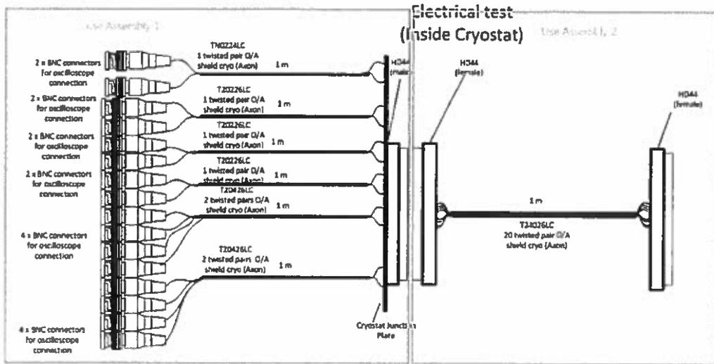
Run Electrical testing separately for matrix of T20226LC & T24026LC and matrix of T20426LC & T24026LC.
