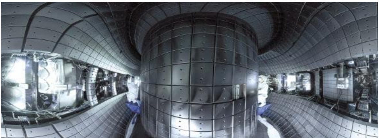
Inside the 'KSTAR' vacuum vessel of the superconducting nuclear fusion research device
