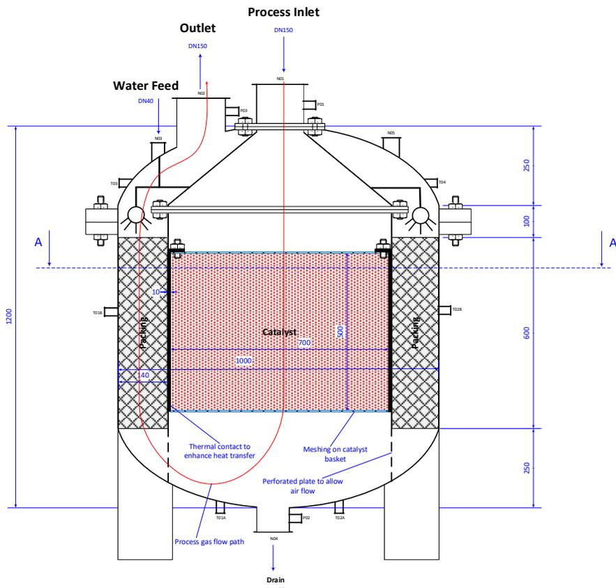
Figure 5: Annular configuration with annular scrubbing section
