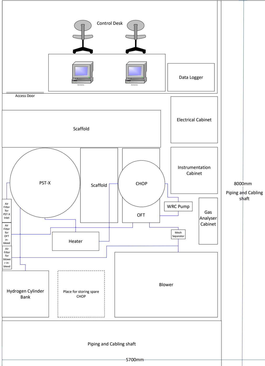
Figure 8: Plan of proposed CHOP qualification facility
