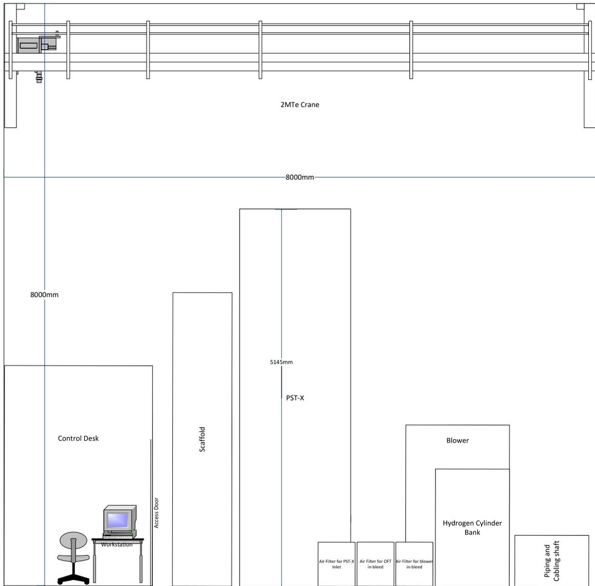
Figure 9: Elevation of proposed CHOP qualification facility
