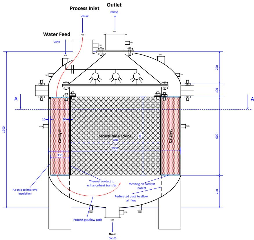
Figure 4: Annular configuration with cylindrical scrubbing stage
