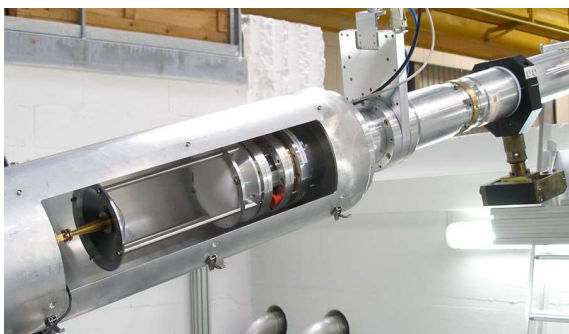
Figure 1: Lens horn connected to a transmission line input (left) and measured beam pattern after 94 m transmission line and 7 miter bends (right).
